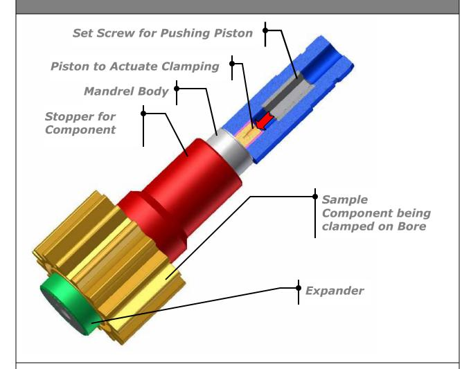
*ITC* make Hydraulic Expanding Mandrels provide EXTREMELY precise clamping due to very large forces developed by a system of hydraulic actuation.
